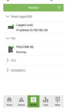
**Step 5** Choose **PID** on the device monitoring screen to access the main menu screen of the PID module, as shown in Figure 6-13.
